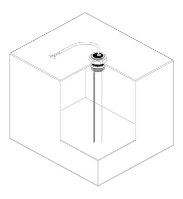
For remote level measurement, the **tank electrode** is installed directly at the tank. It is suitable for:
