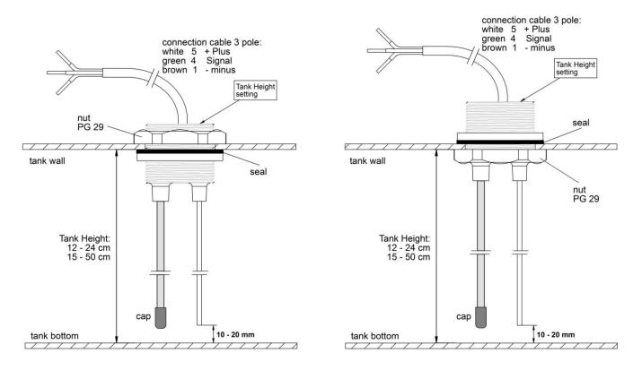
After that, the two stick probes must be cut to identical length (metal saw, strong side cutter, bolt cutter).
