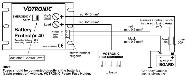
This type of switching allows an effective remote control of the unit by means of a switch being located in the living area. Since the load of the switch is very low (0.002 A), an execution as microswitch is sufficient.
