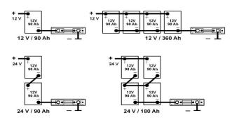
Any battery current should flow over the smart shunt. Therefore, it is to be installed directly near the battery (batteries). Correct calculation of the actual battery capacity is only possible, if all currents are detected correctly by the smart shunt.
