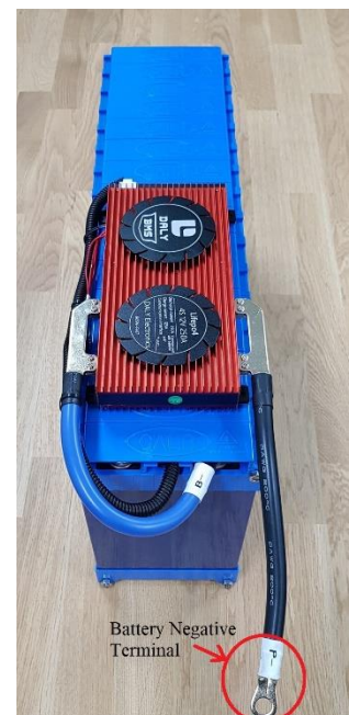
Figure 1- Battery Negative Terminal
