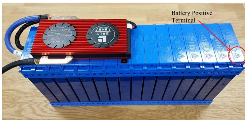
Figure 2 - Battery Positive Terminal
