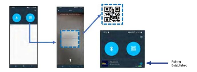
The Bluetooth Monitoring System provides point to point connection. Only one battery can be connected to one device at a time. If more than one battery is configured in series or in parallel, each battery can be checked in turn, one by one, on the same smart device. Simply follow the pairing/connection process for each individual battery.
