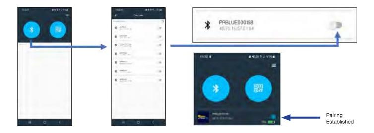
b. Scan the QR code on the battery and the battery Bluetooth ID will appear:
