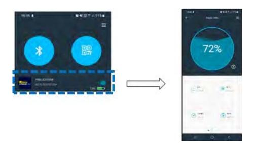
b. Swiping across from the Basic Info screen will show the '**Details Info**' screen. This screen shows battery voltage, battery current, estimated run time, individual cell voltage, battery temperature and battery cycle count.
